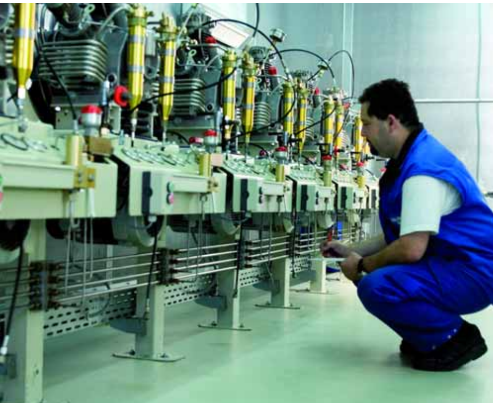
Every BAUER compressor undergoes a rigorous and comprehensive operational test
