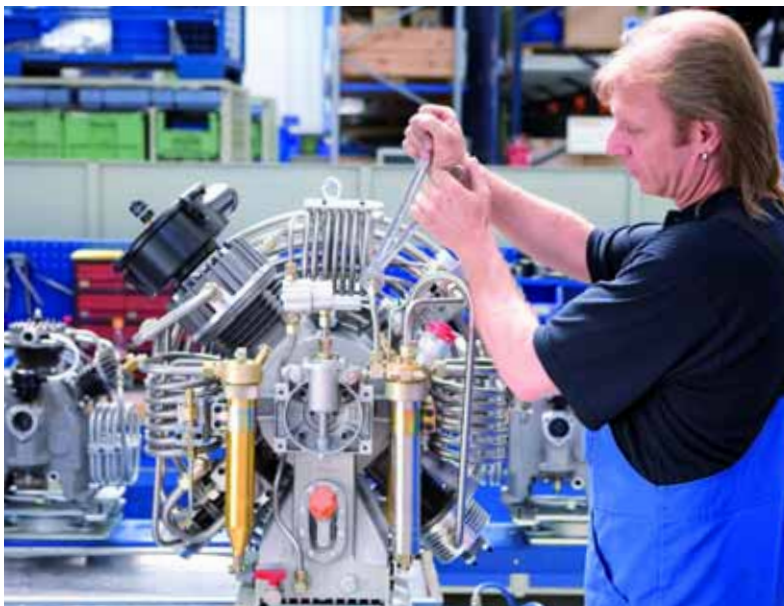
Assembly of a IK 18.1 compressor block
